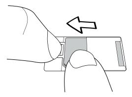
4. Slide the SIM card out from the SIM card slot.
