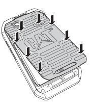
4. Press and hold the bottom of the back cover and slide the back cover latch to the left to the lock the back cover.
