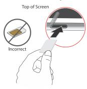
Note: If the card is not inserted correctly, the device will not detect the SIM card. Re-orient the card back into the slot if the SIM is not detected.
