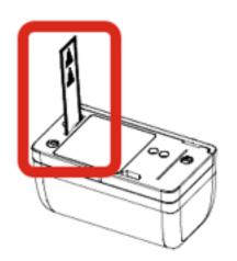
Pull the exposed plastic tab from the Door/ Window Sensor. 5. Once the Door/Window Sensor is detected you will see the **Sensor** icon, and **Pairing...** will appear.
